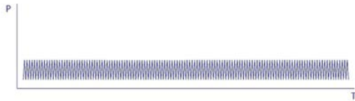
Fig.15 Ventilation with PULSE
